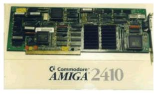
Here you can find some of the information I've found surfing around the internet about the A2410 Card. Apparently this card has been created to fill the need of higher resolution and more colors for the Amiga Unix. The card is based on the TI TMS34010 Graphics Co-Processor running at
