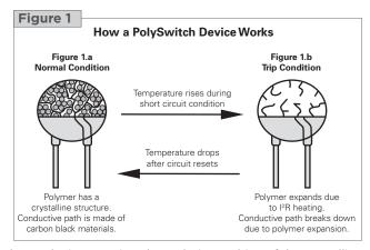
temperature, the crystallites in the polymer melt and become amorphous. The increase in volume during melting of the crystalline phase separates the conductive particles resulting in a large non-linear increase in the resistance of the device.
